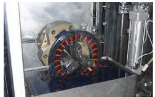
Roll Coating is performed in enclosed and fire protected viewing areas.
