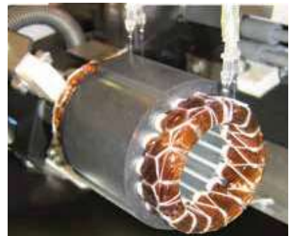
Trickle Systems are either single or dual sided fixtures. Resin coating can be continuous flow or precisely controlled using robotic actuation.
