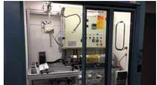
HeatTek Lab unit includes induction, infrared, resistance heating along with Trickle and Roll Coating of test parts.
