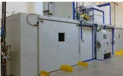
Palletized loads of transformers are cured and processed inside of enclosed vented chambers.
