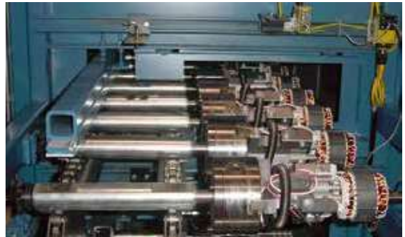
HeatTek Trickle Coat Systems are designed for stators, rotors and armatures and are sized to meet production line volumes and varying product sizes.
