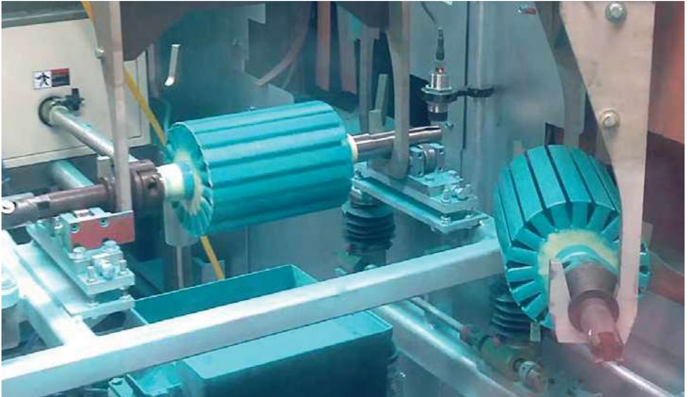
Fluidized beds are used to provide and deliver controlled amounts of powder to preheated parts allowing for controlled film build.
