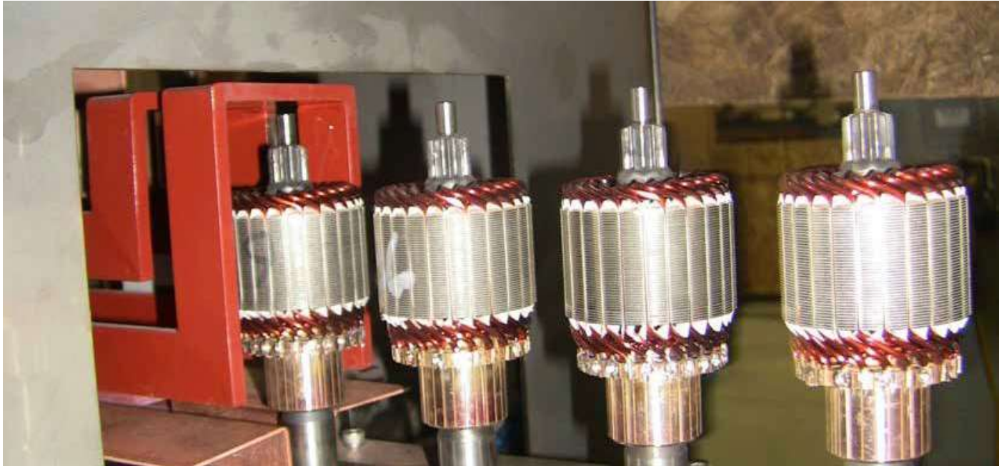
Armatures being heated by a water cooled induction coil.
