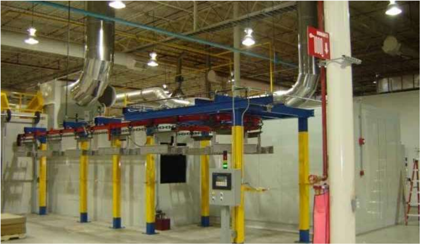
Dip and Bake Systems utilize different conveying methods and transfer single or multiple parts at a time. Conveying Systems are most often designed to index on timed intervals.
