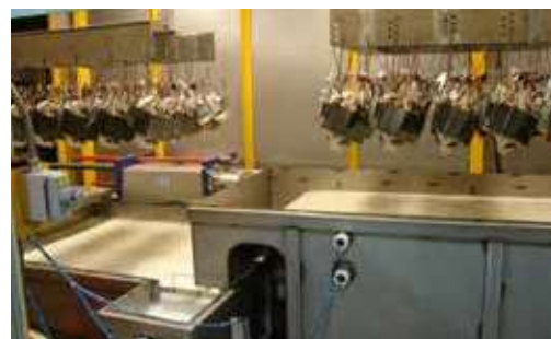
Dip and Bake System utilize all types of resin. Auto fill and control systems are included in all Dip and Bake Systems.
