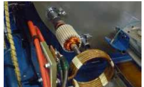
Armature pre-heated via a moving induction coil
