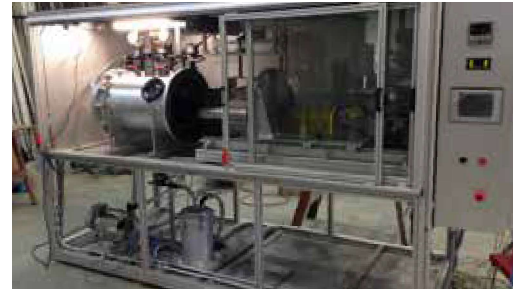
Vacuum coating of parts and IR curing is featured in this particular lab unit.
