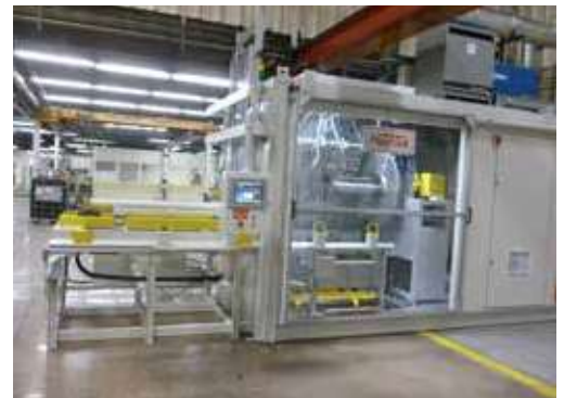
Roll Coat Systems feature multiple heating methods including resistance and infrared heating
