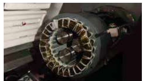
Stator heated / cured using the infrared heating method
